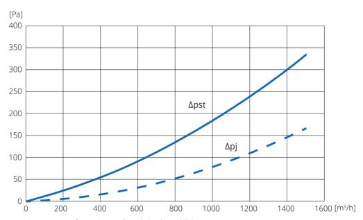
$\Delta pst$  – constant flow resistance through the channel [Pa]  $\Delta pj$  – unit flow resistance per one metre of the channel [Pa/m]
